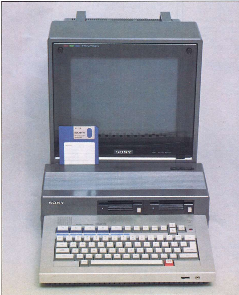
The Sony SMC-70 microcomputer, featuring 3½-inch micro floppy disk drives.
